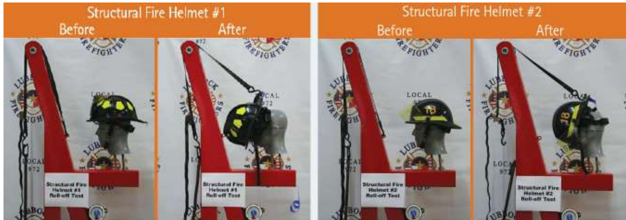
Figure 2. Helmets Before and After the Roll-Off Tests Were Performed
