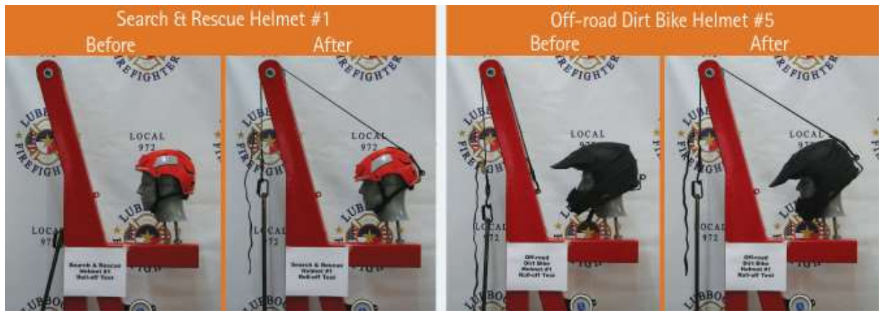
(Left) Search and rescue helmet #1 performed well, rotating only a few degrees forward. (Right) Off-road dirt bike helmet #1 performed satisfactorily, rotating forward slightly more than the previous two helmets.
