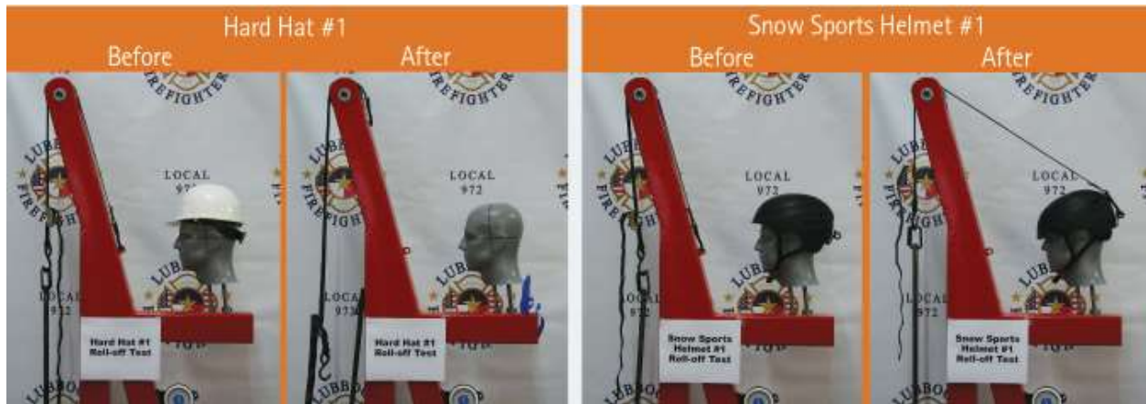
(Left) Hard hat #1 came completely off the head form. (Right) Snow sports helmet #1 performed well, rotating only a few degrees forward.
